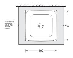
NOTE: BASIN MAY BE SEALED TO COUNTER TOP USING ACETIC CURE SILICONE SEALANT DO NOT USE EPOXY ADHESIVES
